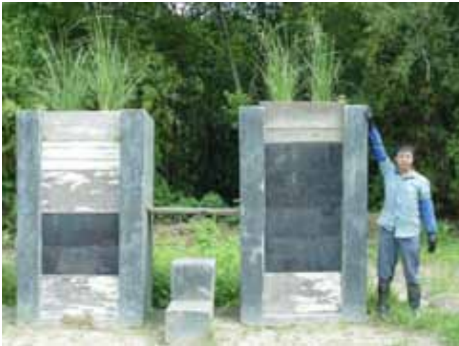
Fig. 4 Cement growing boxes used to investigate the growth of vetiver roots
