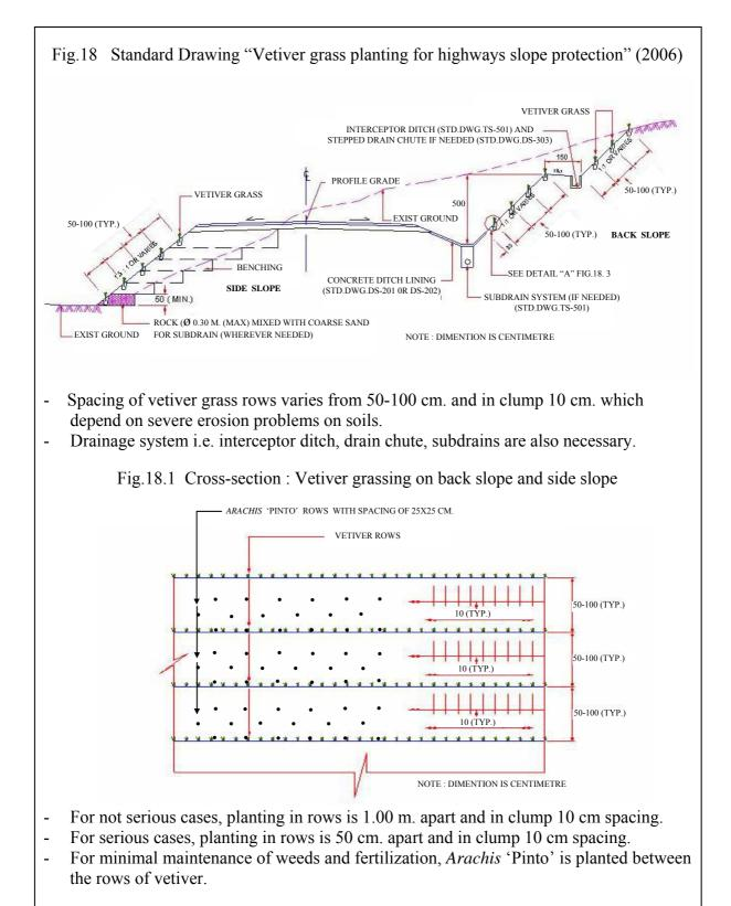
Fig. 18.2 Plan : Vetiver grassing on back slope and side slope
