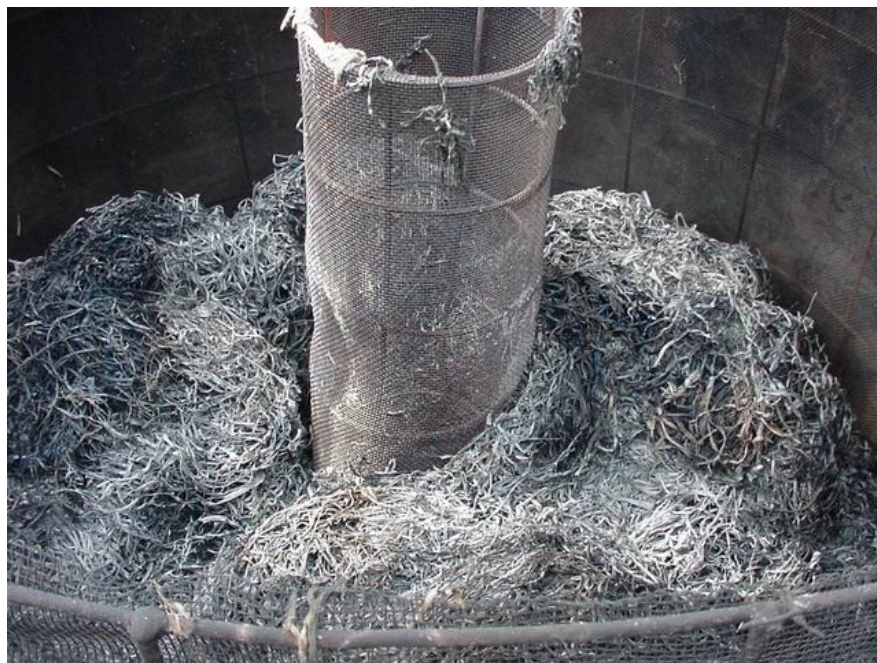
Figure 2. Vetiver Grass Ash before Grinding
