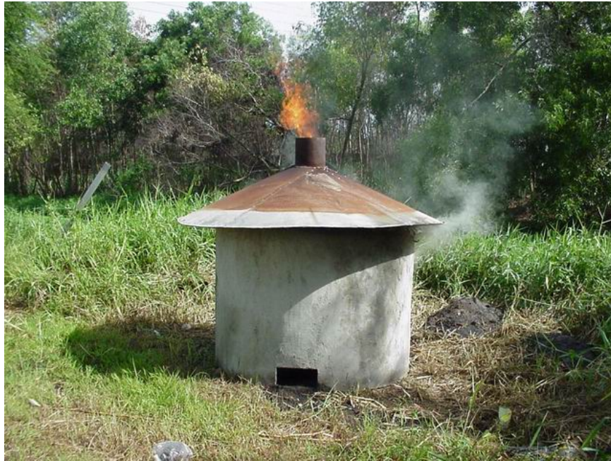
Figure 1. Burning Vetiver Grass by Ferrocement Incinerator
