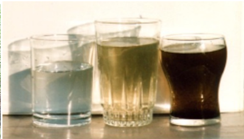
Photo 7. Vetiver filtered effluent, L to R, tap water, Vetiver treated effluent, untreated effluent
