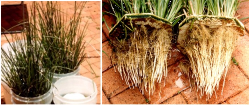
Photo 3. Trial 1, hydroponic Vetiver treatment of effluent
