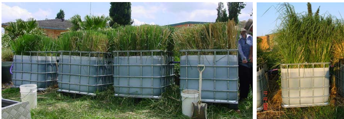
Photo 5 Trial 3, hydroponic Vetiver treatment of effluent, left, cut back at the start of the trial and right, vetiver growth after trial period
