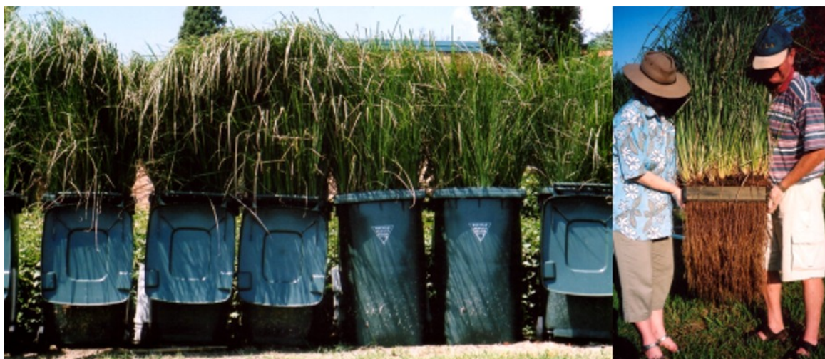
Photo 4 Trial 2, hydroponic Vetiver treatment of effluent
